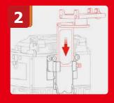
Insert into the base and tighten
