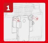
Use the screw to fix the base
